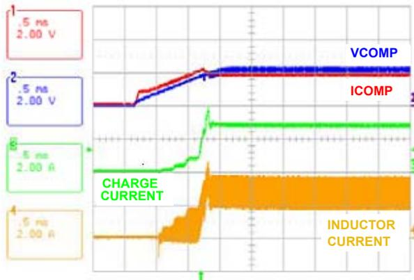
FIGURE 7. CHARGE ENABLE
