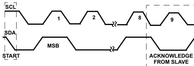
FIGURE 17. ACKNOWLEDGE ON THE I<sup>2</sup>C BUS
