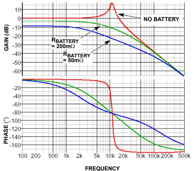
FIGURE 24. FREQUENCY RESPONSE OF THE LC OUTPUT FILTER
