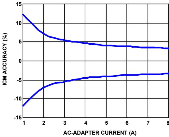
FIGURE 5. ICM ACCURACY vs AC-ADAPTER CURRENT
