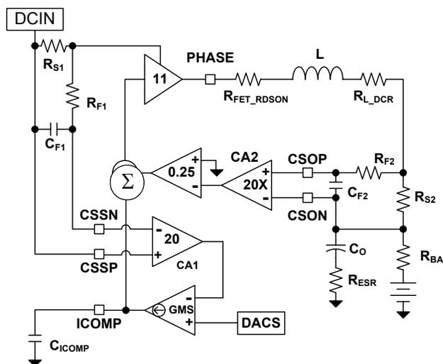
FIGURE 22. ADAPTER CURRENT LIMIT LOOP
