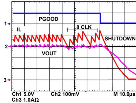
FIGURE 40. OVERCURRENT PROTECTION
